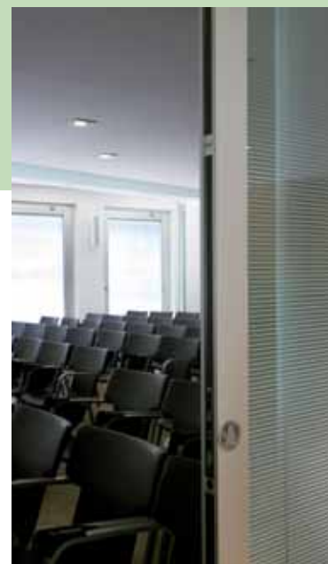
Parete manovrabile insonorizzata, di grandi dimensioni, in un unico elemento, traslabile parallelamente a se stessa/Movable one-piece sound-insulated wall of large dimensions which slides across to position itself on a second guide parallel to the first
