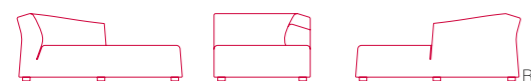
CHAISE LONGUE MODULE R AND L L103 D175 H72 seat D71 H38
